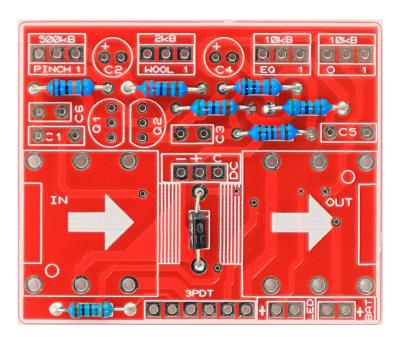
Place the resistors and diodes. If you have troubles reading the values, check out our <u>"Reading Part Values"</u> tutorial.
